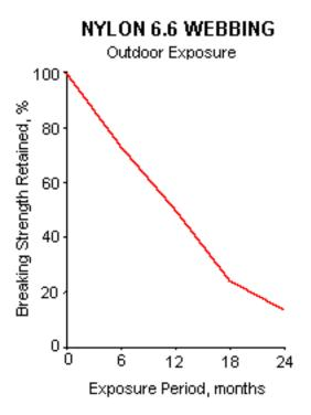
With this kind of rapid deterioration, it is obvious why replacing the webbing every two years is essential to driver safety. Old and weakened belts could easily snap under the loads imposed upon them in an accident situation. Failure to properly restrain the driver in a crash would have devastating consequences.
