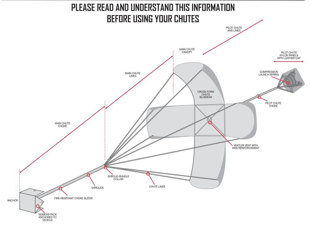
**MOUNTING)** The pilot chute is the anchor that pulls the canopy out for deployment. For the drag chute to deploy properly, the pilot chute must launch into clean, undisturbed air. Mount the pack in a position and angle that assures clean air deployment.
