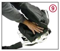
4) Lay chute on ground and fold in half lengthwise. Fold in half lengthwise again. Walk chute back to the vehicle in this position.
