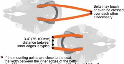
should be equal to or 1" less than the width of the HANS collar
