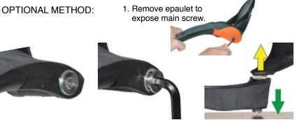
2. Loosen main screw minimum 1/4" (6mm).
