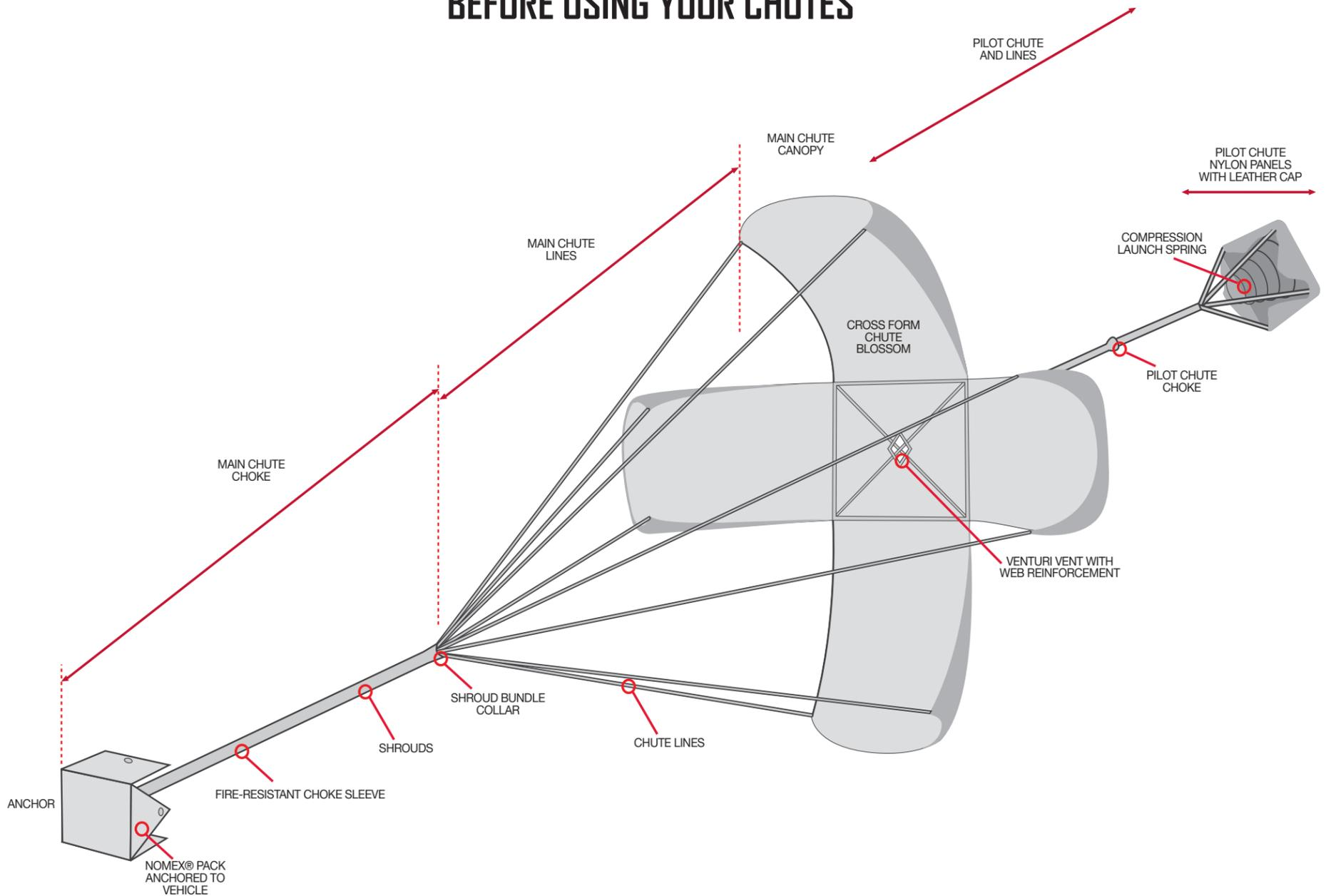
**MOUNTING)** The pilot chute is the anchor that pulls the canopy out for deployment. For the drag chute to deploy properly, the pilot chute must launch into clean, undisturbed air. Mount the pack in a position and angle that assures clean air deployment.
